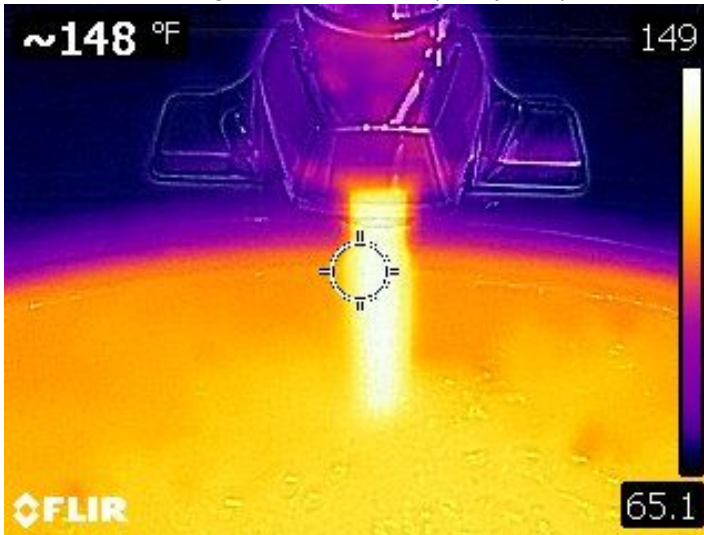
Garage water heater has output temperature too high at 148 degrees F. measured at master bath sink faucet - extreme hazard (See photo & scald chart)
